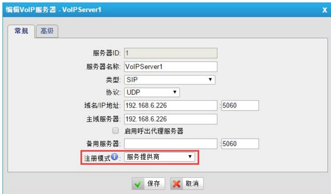
The screenshot shows the '编辑VoIP服务器 - VoIPServer1' configuration window. The '常规' (General) tab is active. The '注册模式' (Registration Mode) dropdown menu is highlighted with a red box and set to '服务提供商' (Service Provider). Other fields include: 服务器ID: 1, 服务器名称: VoIPServer1, 类型: SIP, 协议: UDP, 域名/IP地址: 192.168.6.226:5060, 主域服务器: 192.168.6.226, 备用服务器: :5060, and '启用呼出代理服务器' (Enable Outgoing Proxy Server) is unchecked. '保存' (Save) and '取消' (Cancel) buttons are at the bottom.
